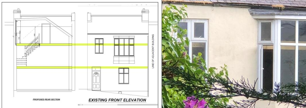
The drawing is our own approximate annotation over the applicant's submission showing how the floor positions might run through to the frontage, the photograph clearly shows the negative impact of the floor cutting through the bay and window.
